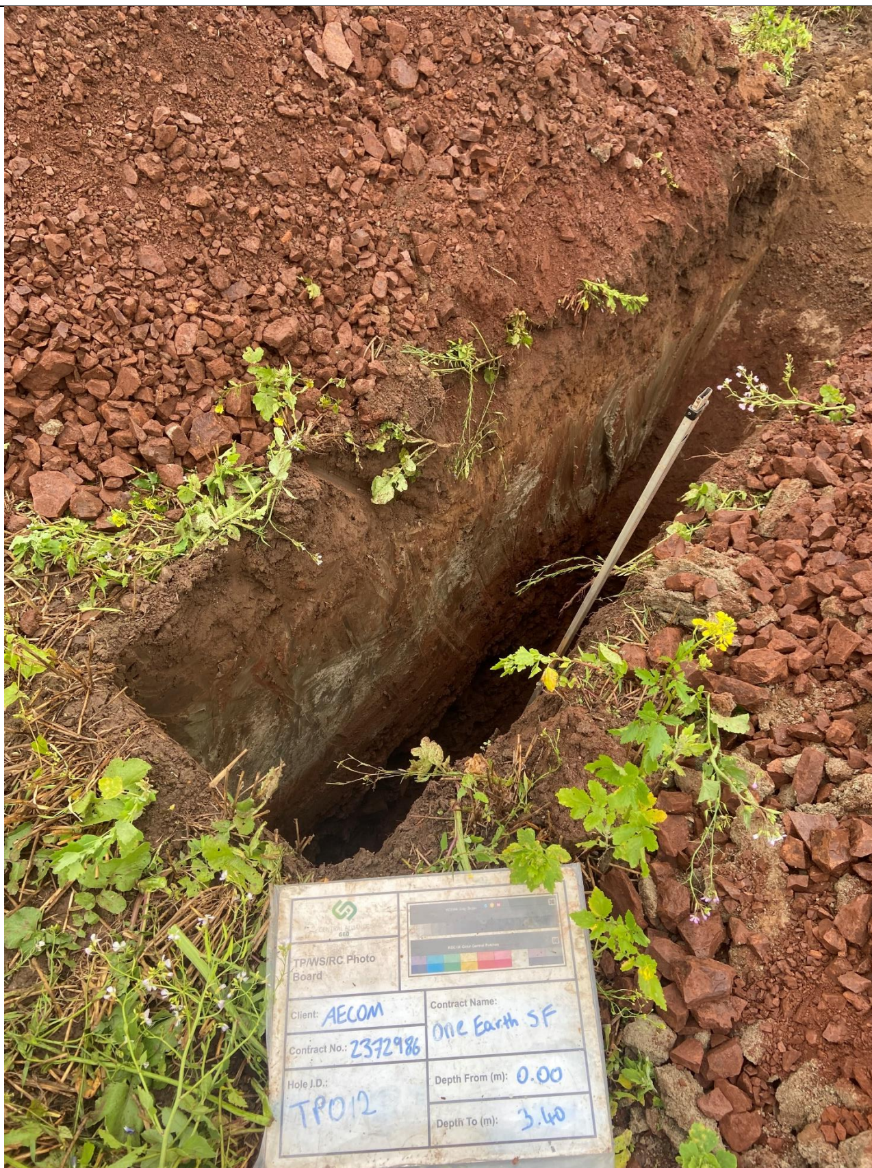
PHOTOGRAPH 3 – TP012 – 0.00m to 3.40m bgl
