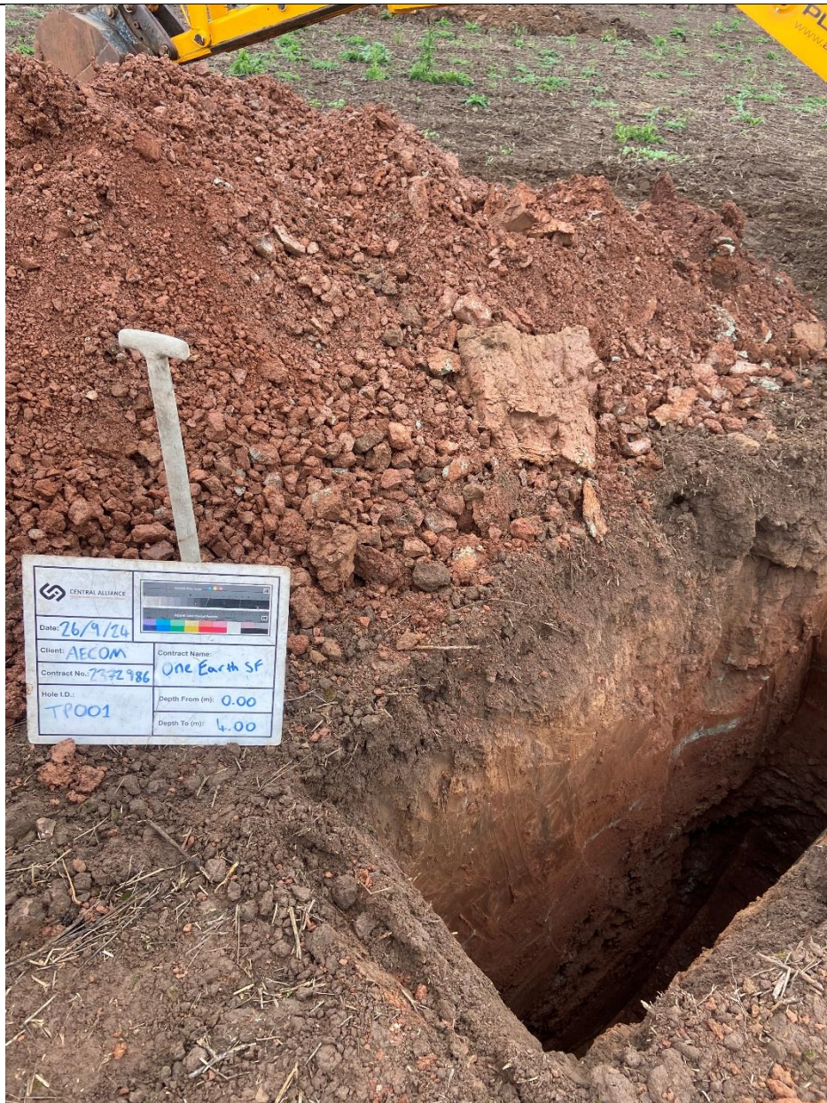
PHOTOGRAPH 2 – TP001 – 0.00m to 4.00m bgl
