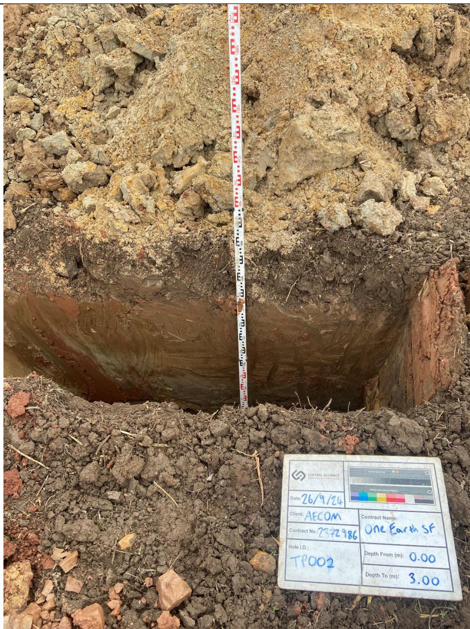
PHOTOGRAPH 1 – TP002 – 0.00m to 3.00m bgl
